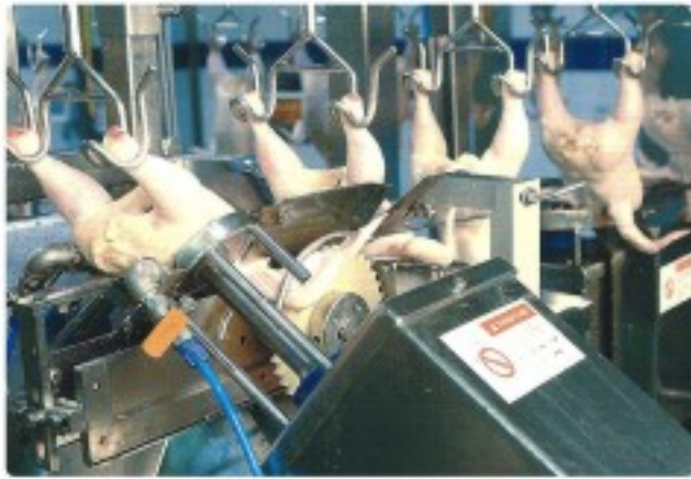
Wing cutter Separating the wings from the carcass through two rotary blades
