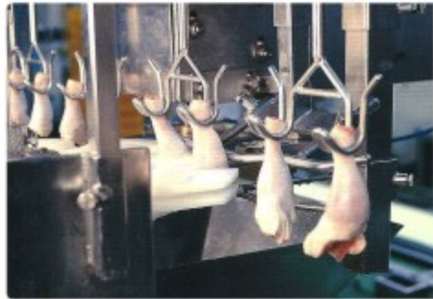
Thigh cutter Thigh cutter is the machine cutting the thigh under the drum stick and the rotary blade cuts the joint.
