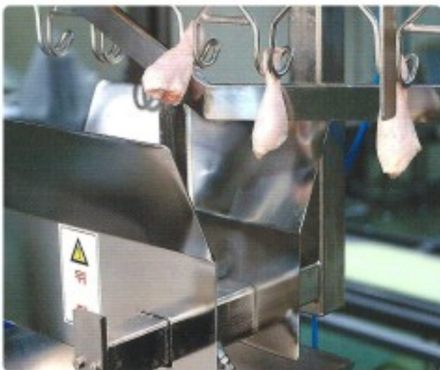
Drum-stick dropper Playing the role of dropping the drum stick from the shackle, as the final processing of cut-up system, after all of the cut processing have been finished
