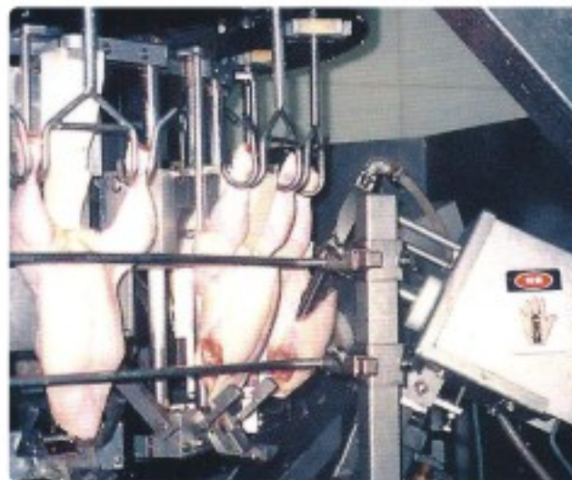
Mastodon bone cutter Consisting of two rotary blades, with the first blade incising the skin between legs and breast and the second blade cutting subsequently the front part (the remaining part)
