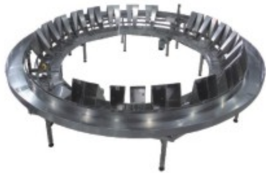
Gender identify turntable with 20 work positions (5.6 meters in diameter)
