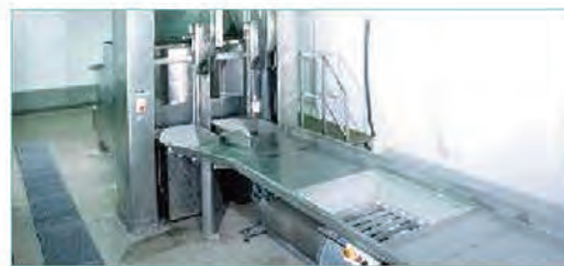
■ Paunch & manifold process line with waste transfer, which is used for fertilizer, elevator, scalding cleaner and defatter 大肚 & 肚加工线, 包括废弃物 (可做肥料) 吹送, 提升机, 淋烫清洗机和除脂机
