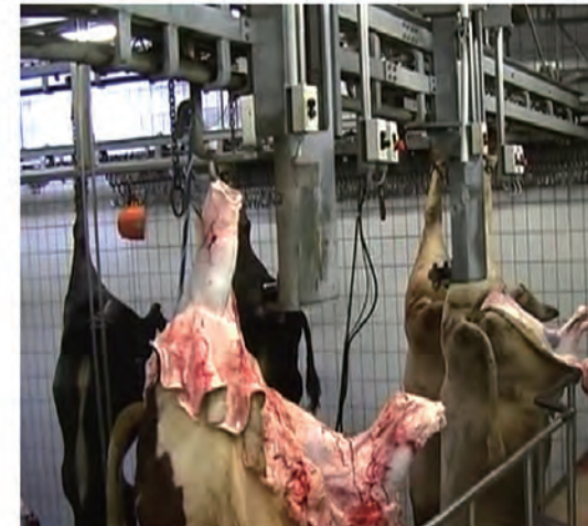
▲ 3 pneumatic hook up rail, capacity 75 ph 3副气动挂钩轨道系统, 产量75头每小时
