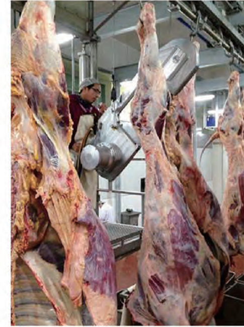
Splitting half manually 胴体手工劈半
