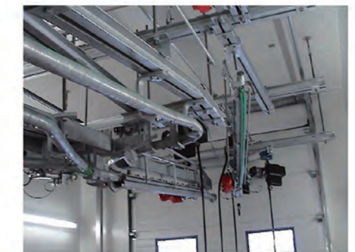
Carcass dispatch system with empty hook receiving element 胴体发货系统, 含空钩接收单元
