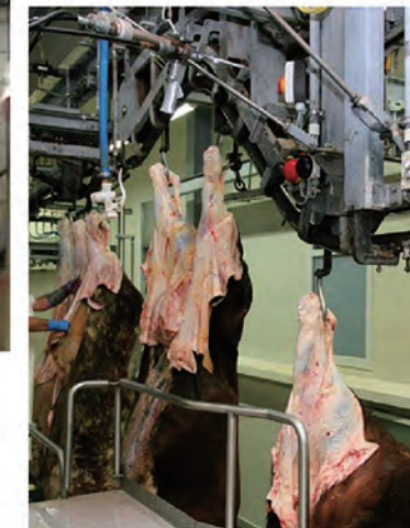
▲ Electric chain elevator, capacity 120 ph 电动链条式提升机, 产量120头每小时
