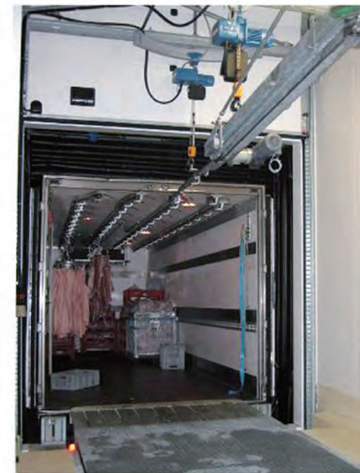
Telescopic loading arm with elevator for carcass dispatch 胴体发货汽车接轨器, 含提升机
